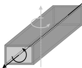
FIG. 2: Vizualisation of a bar rotation along its hozirontal axis (black) and vertical axis (light grey).
