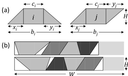
FIG. 1: (a) Bars variables ; and (b) two example of packing 4 bars with different 180° rotations and flips (figure from [2])
